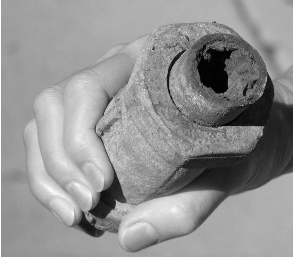
FIGURE 8.12 This 10-year-old water supply pipe has accumulated mineral deposits that make its internal surface rough.
