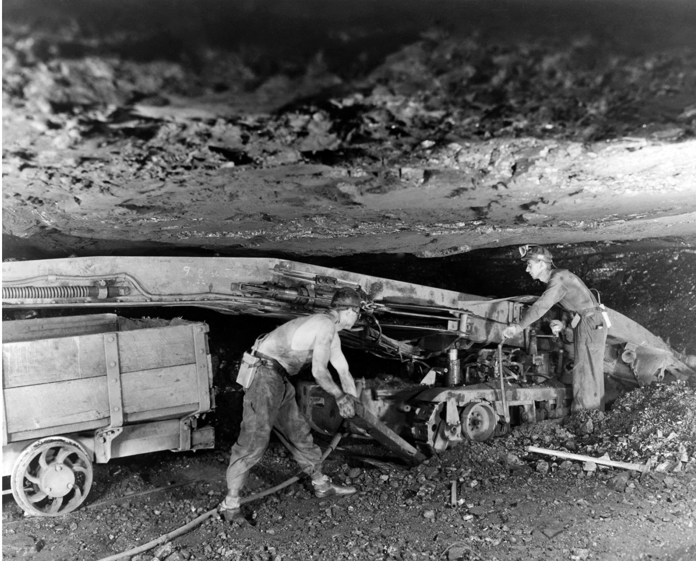
FIGURE 7.3 U.S. coal miners, circa 1930–1960, wear no respiratory protection as they operate a mechanized coal bin loader.
