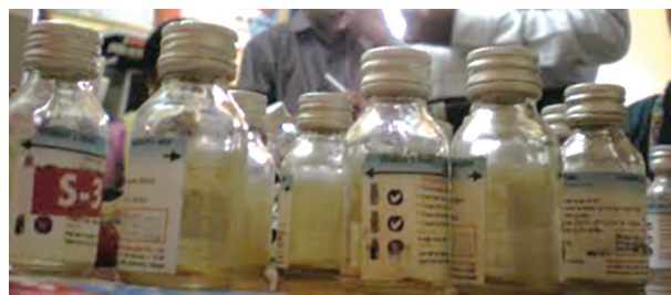
FIGURE 3. H_2S testing vials. Ready for distribution to citizen-scientists who will self-manage sampling.
