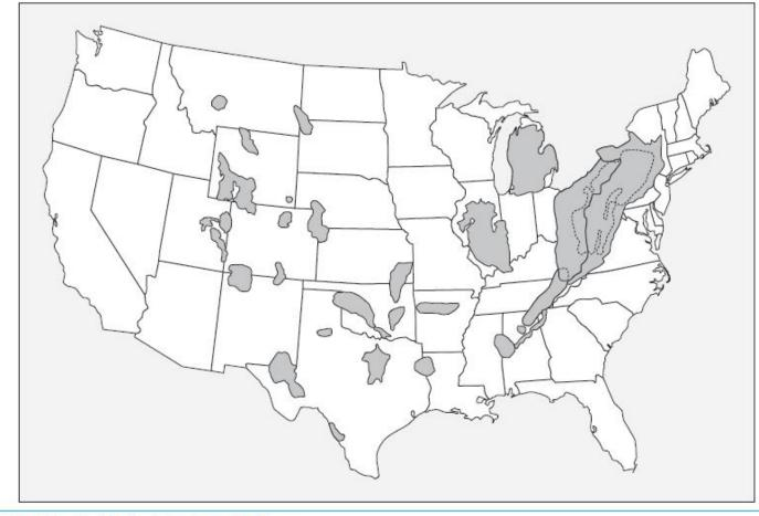
FIGURE 4.2 Shale basins in the lower 48 U.S. states.
