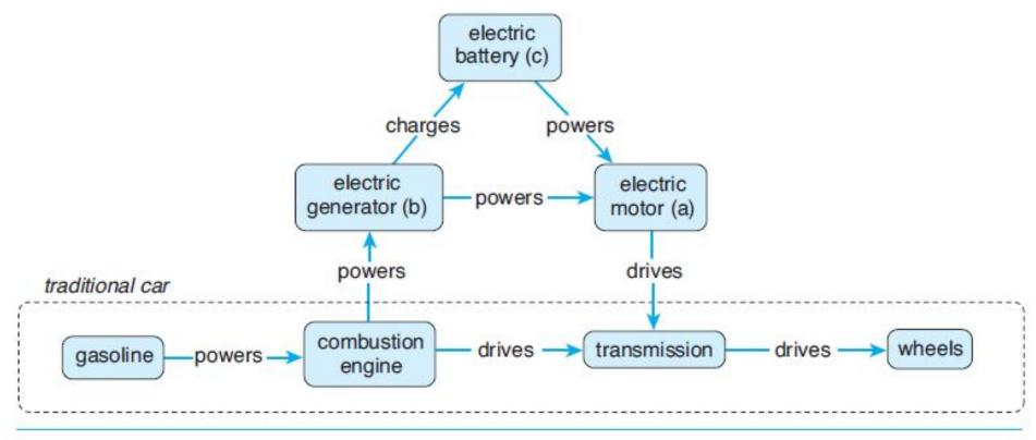
FIGURE 4.17 Schematic configuration of a hybrid car.
