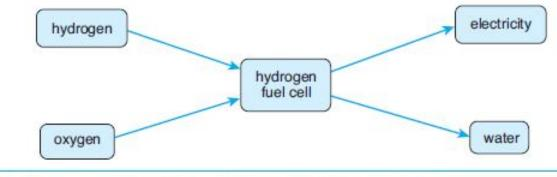
FIGURE 4.21 A conceptual model of a hydrogen fuel cell.
