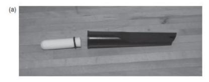
Figure 2.13 Area monitoring: A filter inserted into the nozzle of a vacuum cleaner (a) collects dust to be analyzed in a laboratory. Personal monitoring: A portable sampling device (b) incorporates a pump that takes a continuous air sample near the subject's breathing zone; the device also collects a sample of particulate matter over the whole period.
